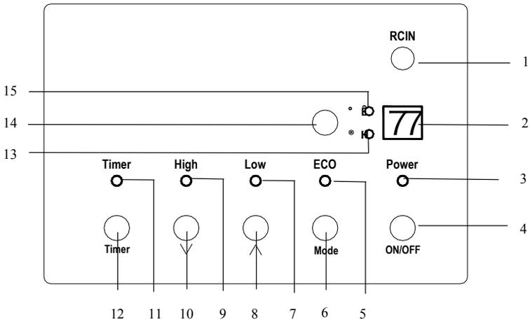
01. Signal receiving window: For receiving remote control signal.
